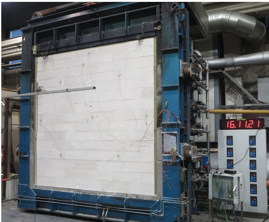
Figure 2. Unexposed side of the fire test prior to the fire test.
