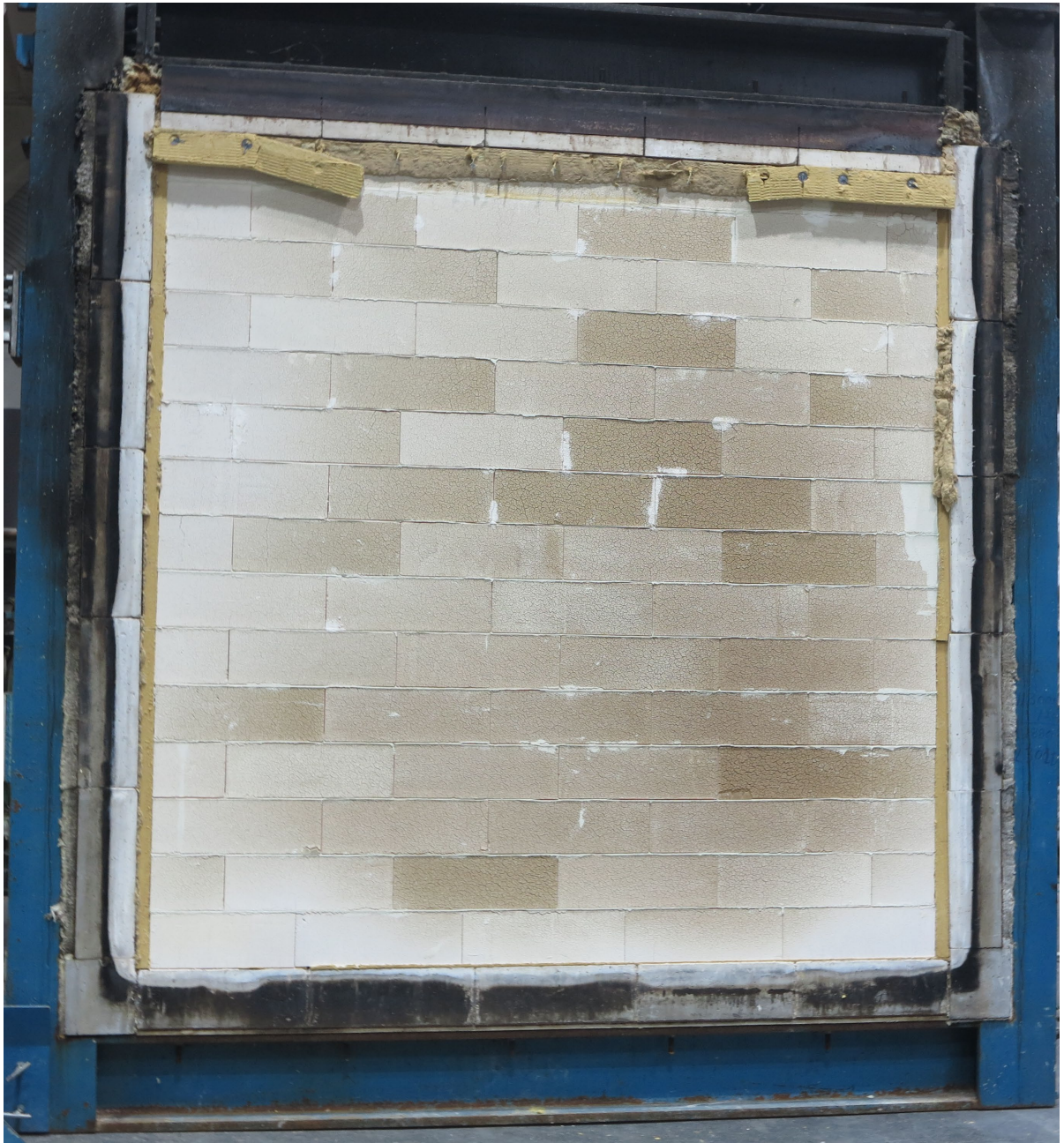
Figure 11. Fire exposed side of the test specimen after the end of the fire resistance test.
