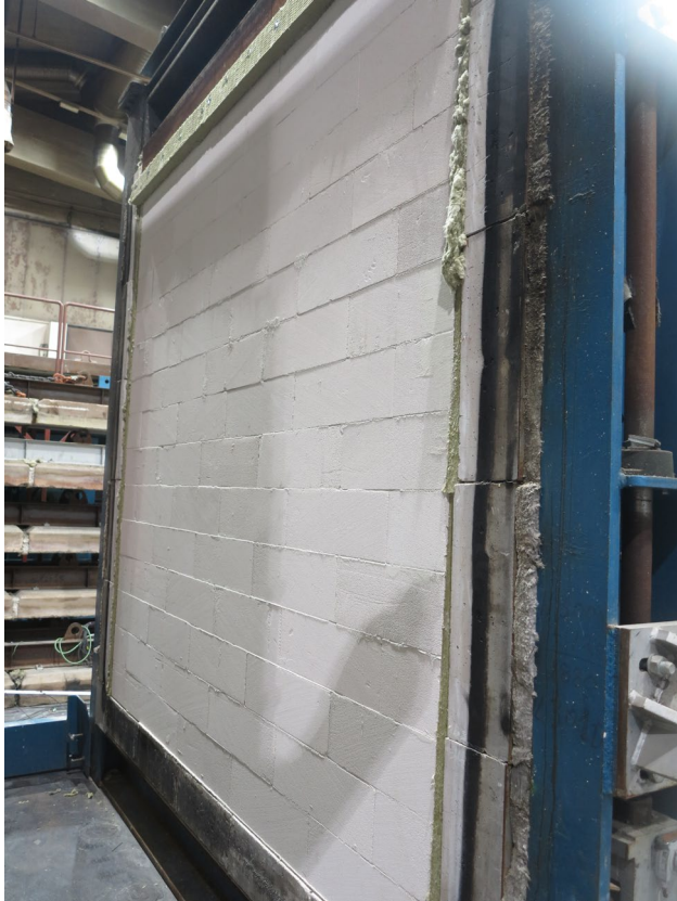
Figure 1. Exposed side of the fire test prior to the fire test.
