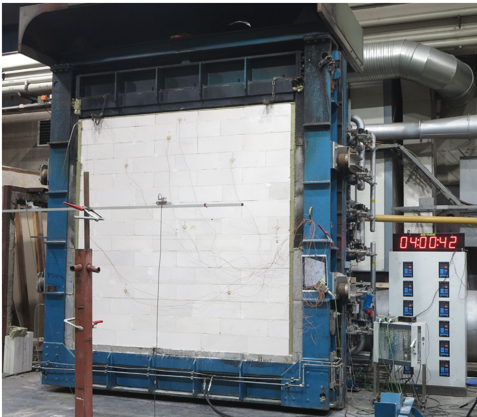
Figure 10. Unexposed side of the test specimen, 12 s after the end of fire resistance test.
